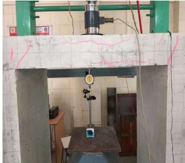
Figure 8- Flexural failure at bottom of slab and shear failure at support.
