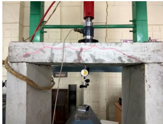
Figure 7- Flexural failure of slab
